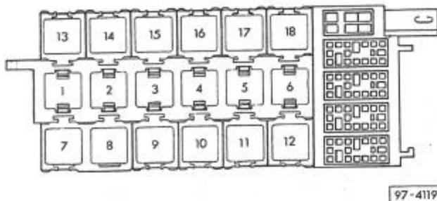
**4** - Buzzer for side lights and radio
